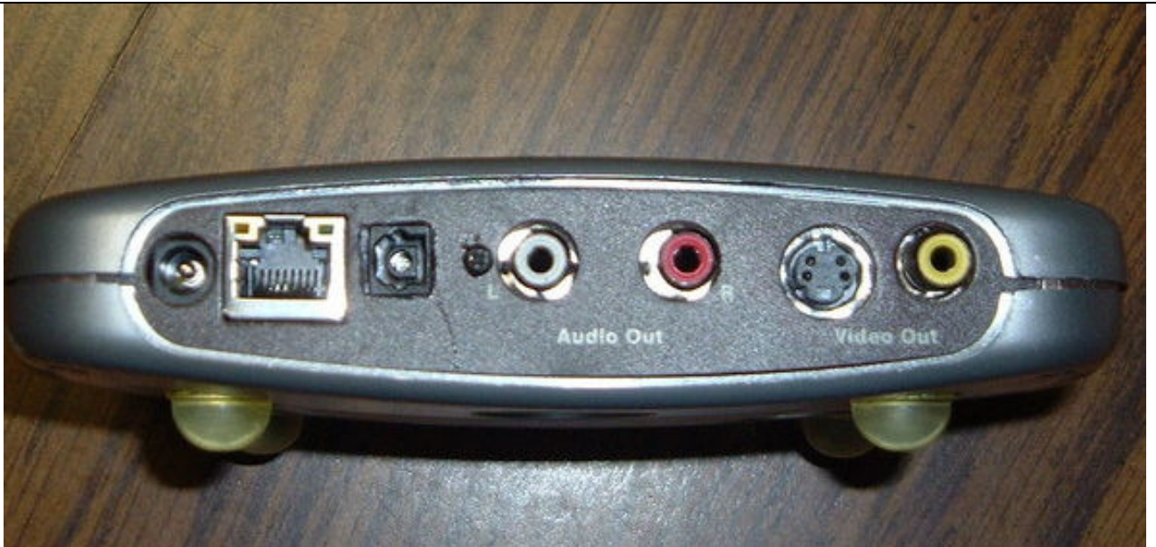
Fig 13a: TOSLINK Position in a RCA MediaMVP – External View
