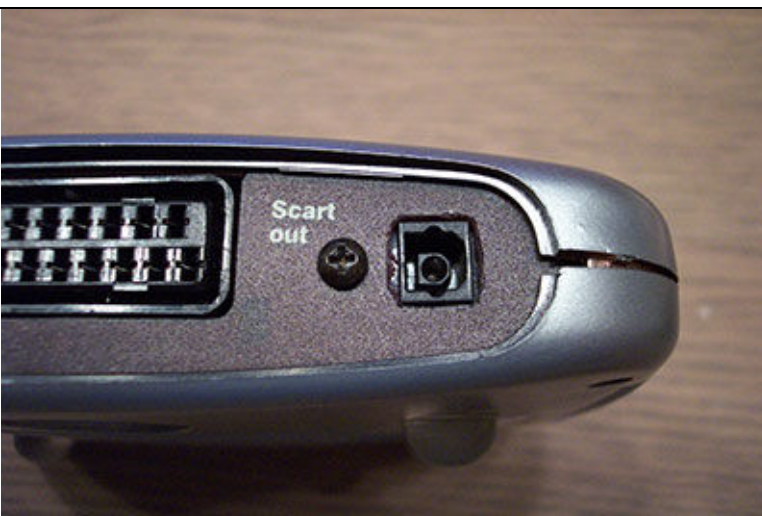
Fig 12a: TOSLINK Position in a SCART MediaMVP – External View
