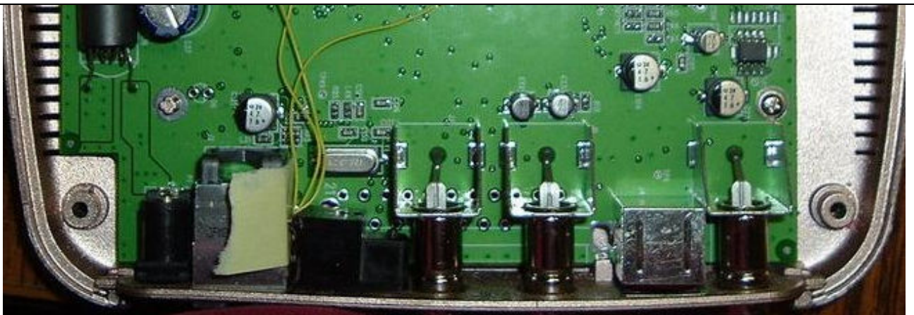
Fig 13b: TOSLINK Position in a RCA MediaMVP – Internal View
